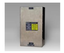
Our Signal Filters are supplied in a compact sized format with current ratings up to 5A AC or 8A DC per phase. The operating voltage is 230V AC or 24V DC per line, and the filter enclosure is constructed of nickel-plated tin. They are available in up to 12-line versions, however further versions are available on request.
